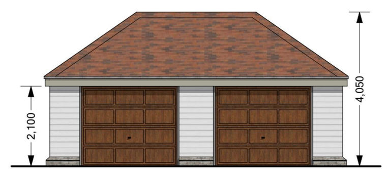
GARAGE NORTH ELEVATION 1:100
