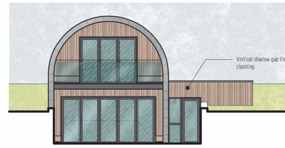
PROPOSED REAR ELEVATION SCALE 1:100 @ A1
