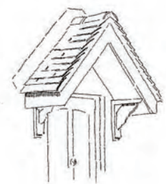
Porch detail with plain clay tiles
